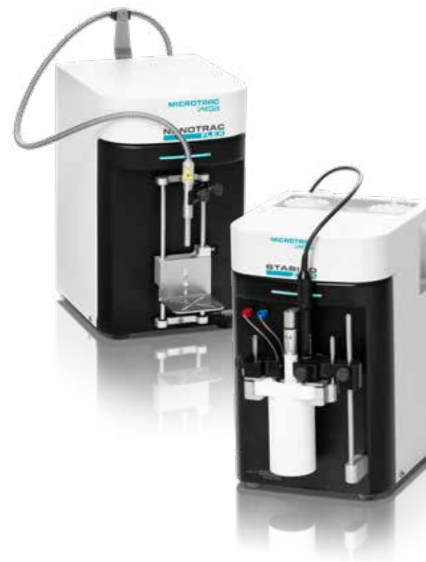
Polyelectrolyte titration of 10 mL P-DADMAC against PVS shown here in streaming potential
